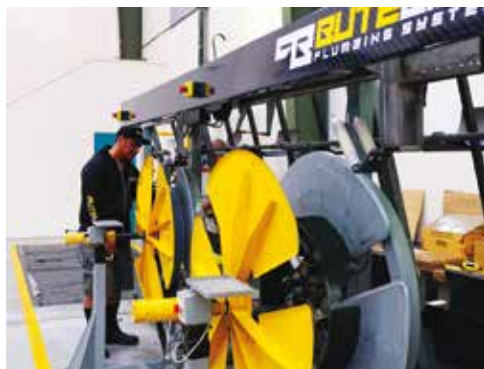
Manufacturing coils on the Buteline Pipewinder
