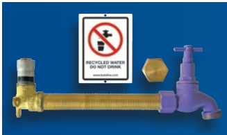
RECYCLED WATER KIT RVVK1 - 5/8" BSP x 20mm x 200mm brass lugged elbow, lilac coloured hose tap, test cap and non-potable supply sign.
