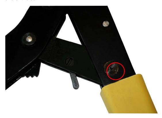
2. Turn the tool over and remove the circlip securing the adjuster cam.
