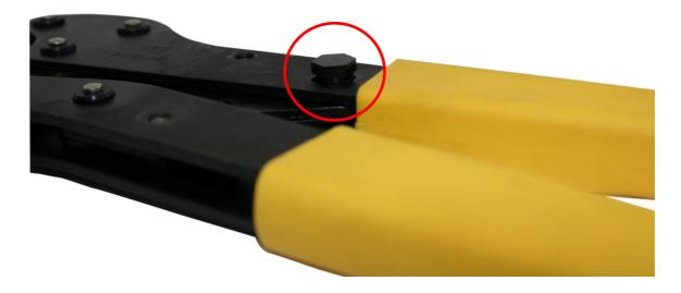
5. Push the hexagonal head of the cam back into the handle and replace the circlip to retain the adjuster cam.
