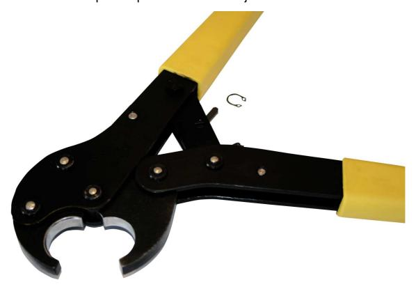
4. Push the adjuster cam out from the circlip side until the hexagon head of the cam disengages from the handle, and turn the cam anticlockwise, so that it is moved around 1 flat of the hexagon.
